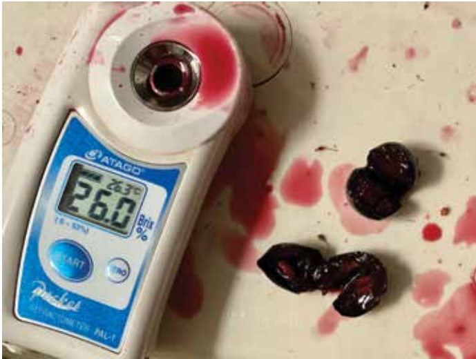
Hand-held digital refractometer is a critical tool to measure sugar in grapes as they ripen—these are purple-juiced Alicante grapes
